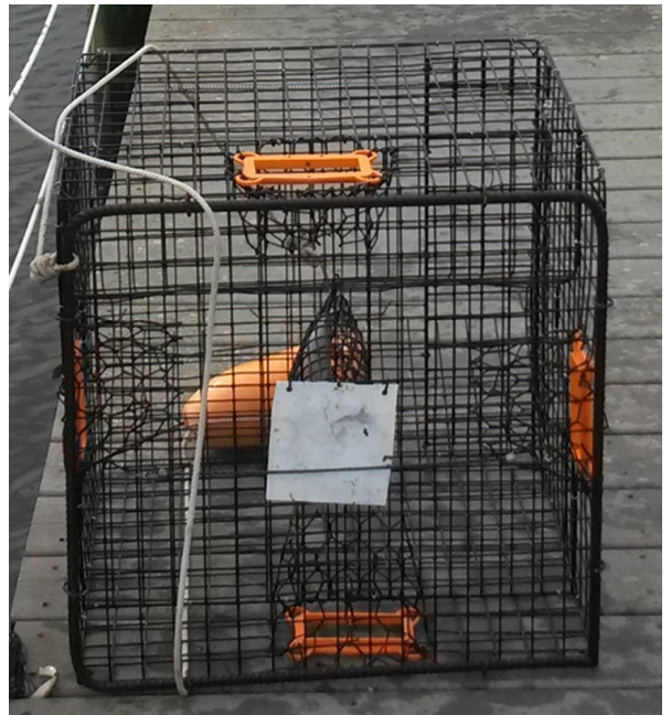
Fig. 7. Commercially outfitted crab pot with BRDs inserted for reference. Crab pot is on its side for a look at the bottom. Notice the rebar frame and line tied at the bottom.
